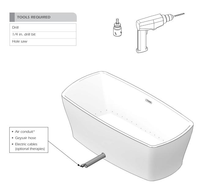
(\*): The location of the air conduit is shown as an example. It may differ depending on the positioning of the remote components and the orientation of the bath.
