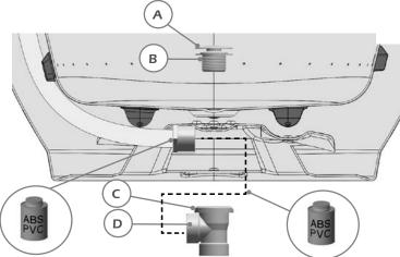
NOTE: If necessary, cut the overflow pipe to the desired length, and glue it to the PVC connector and to the drain.
