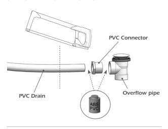
NOTE: If necessary, cut the overflow pipe to the desired length, and glue it to the PVC connector and to the drain.
