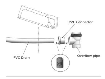
NOTE: If necessary, cut the overflow pipe to the desired length, and glue it to the PVC connector and to the drain.
